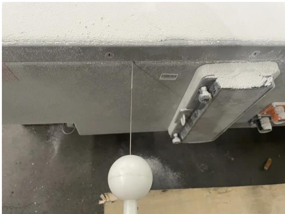
IP6X(Against access to hazardous parts) -1#
