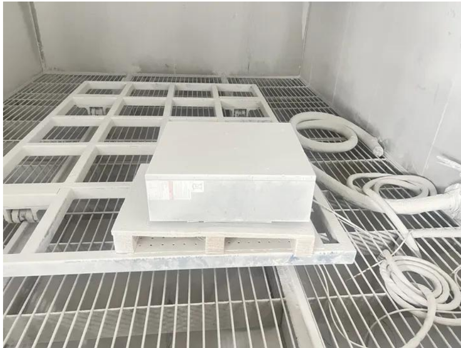
IP6X Setup after test-(Against solid foreign objects indicated)-1#
